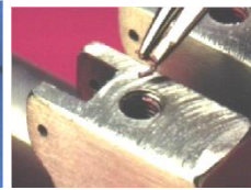
Difficulty in retrieving tangs from blind holes.
