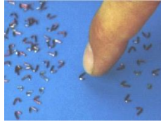
Broken tangs persist at the work site.
